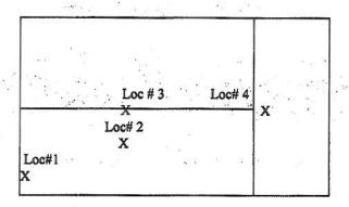
Location # 1 Bottom left corner of Panel Location # 2 Mid-span of bottomPanel Location # 3 Mid-span of Horizontal Scheme Location # 4 Mid-span of Vertical Scheme
